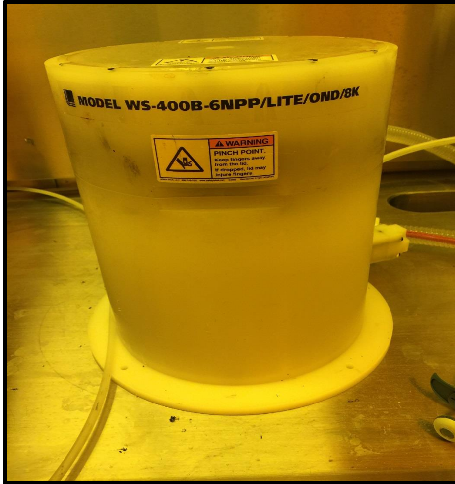
Figure 19: Laurell technologies WS-400-6NPP-LITE spin coater
