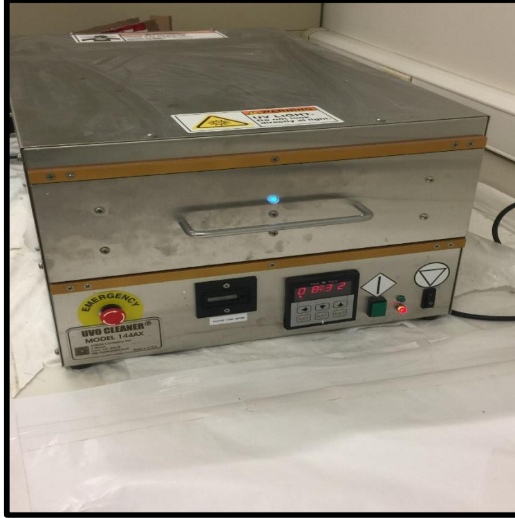
Figure 18: Jelight UVO cleaner-144AX used in this research
