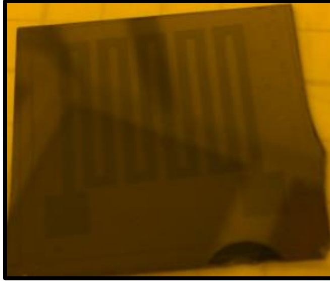
Figure 44: Schematic of SiO 2 substrate after etching photoresist
