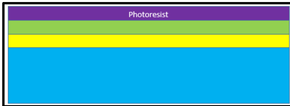
Figure 33: Cross-sectional layout of Silicon substrate with photoresist
