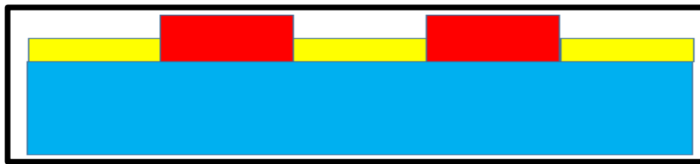
Figure 46: Cross-sectional view after etching nickel (second time)
