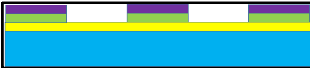
Figure 41: Cross sectional view after etching Nickel
