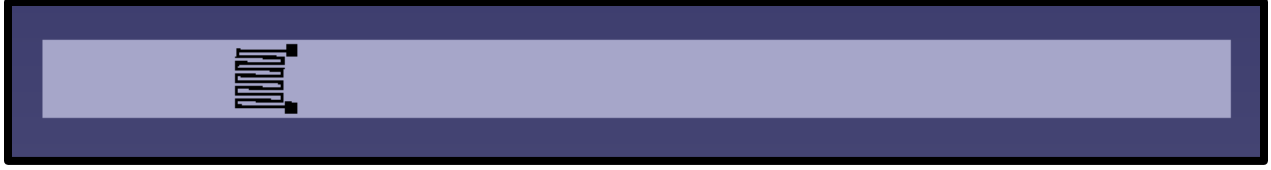
Figure 58: Schematic of CNT-polymer strain gauge on cantilever beam
