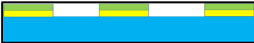
Figure 43: Cross sectional view after etching Photoresist (second time)
