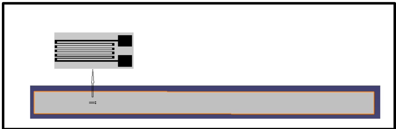
Figure 50: Schematic of strain gauge placed on cantilever beam. Exploded view of the sensor is shown in the inset
