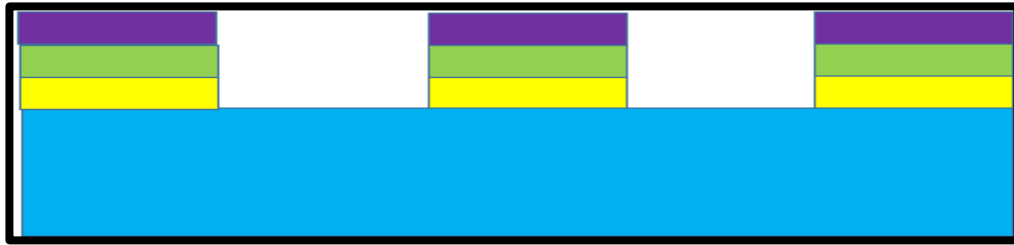
Figure 42: Cross sectional view after etching Titanium
