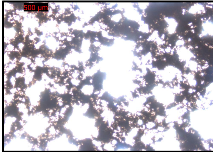
Figure 79: Single layer thin film of 5 wt. % CNT solution deposited on glass substrate
